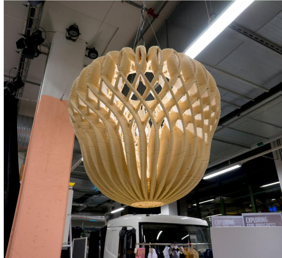
"Lattice Lamp" is made of 3d-printed wood composite. Created by Charlotte von der Lancken and printed at RISE.
